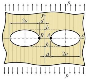
Fig. 1. Scheme of loading the plate with a holes
