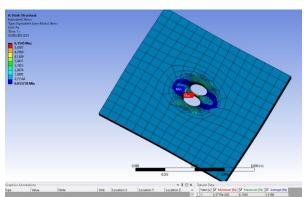
Fig. 10. Relative maximum stresses in the plane with a two circular hole (isotropic material)
