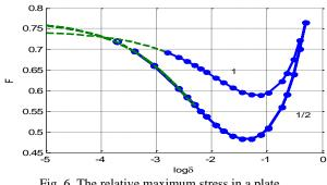
Fig. 6. The relative maximum stress in a plate made of material EF<sub>90</sub>; 1 - circular holes, 1/2 - elliptical holes
