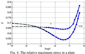
made of material CF1<sub>90</sub>; 1 - circular holes, 1/2 elliptical holes
