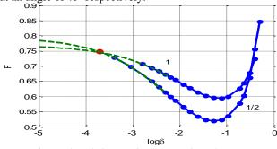
Fig. 5. The relative maximum stress in a plate made of material EF; 1 - circular holes, 1/2 elliptical holes
