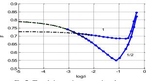
Fig. 7. The relative maximum stress in a plate made of material EF45. 1 - circular holes, 1/2 elliptical holes
