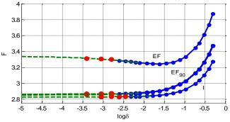
Fig. 9. Relative maximum stresses in the half-plane with a circular hole (EF material end isotropic material)
